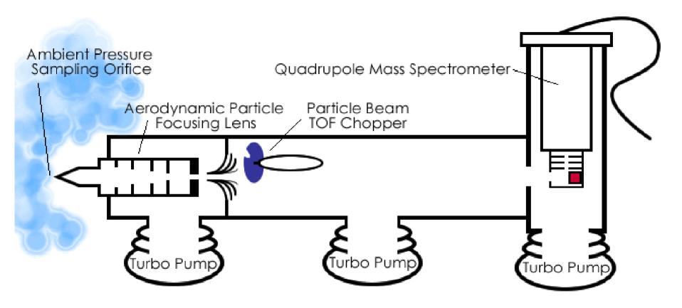
100% transmission (60-600 nm), aerodynamic sizing, linear mass signal.
